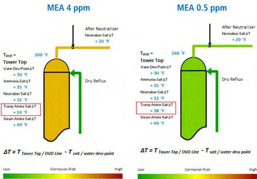
**Figure 1.** Screenshots of the CRM output depict the reduced corrosion risk to the top of the tower by reducing MEA from 4 ppm to 0.5 ppm in the desalted crude.
